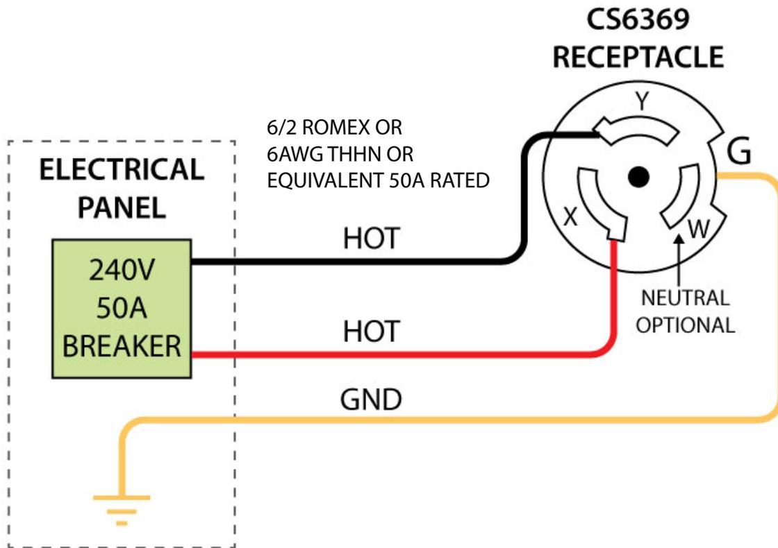
If the Green Machine requires a 220/240V, 50A circuit for charging, install an outlet using a CS6369 receptacle as shown in the diagram above. The neutral wire (W) is not needed by the Green Machine charger and can be left not connected. The neutral wire can be connected if needed for other equipment - it will not affect the Green Machine equipment.
